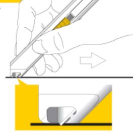
Hold the TS-1 as you hold a pen, and give it enough pressure to leave no space between the TS-1 and a sheet of paper while cutting.
